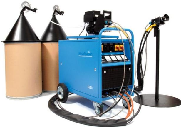
In the Arcspray process, two electrically charged wires are driven and guided so that they converge at a point and form an arc. An air nozzle atomises the molten metal produced from the wire and projects it towards the work piece using high pressure air. This spray solidifies when it hits the surface of the work piece to form a
